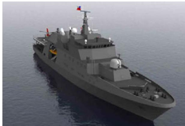
*Danubio IV Project Phase 2 (OPV-80 - Chilean Navy): Building of a maritime zone patrol vessel, similar to OPV 81 "Piloto Pardo" and OPV 82 "Comandante Toro", conditioned for shipping in Antarctic waters and with an extended bridge to facilitate maritime operations.*
